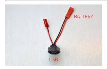
A full charge takes approximately 6/7 hours Inside the charging board there is an LED that turns red during charging and turns blue when charging is complete.
